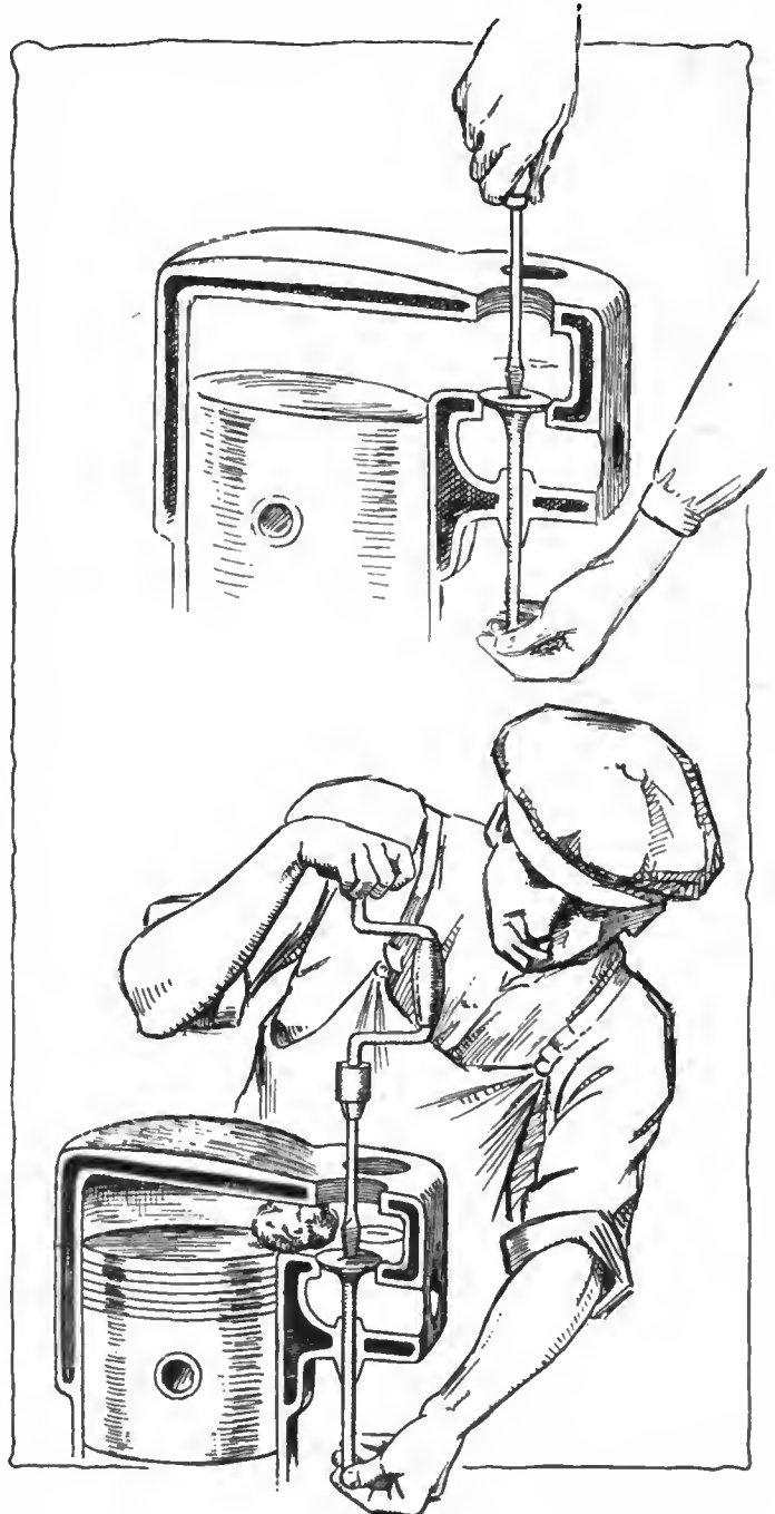
Fig. 3—Grinding work can be done either by a plain screwdriver or a brace and bit
